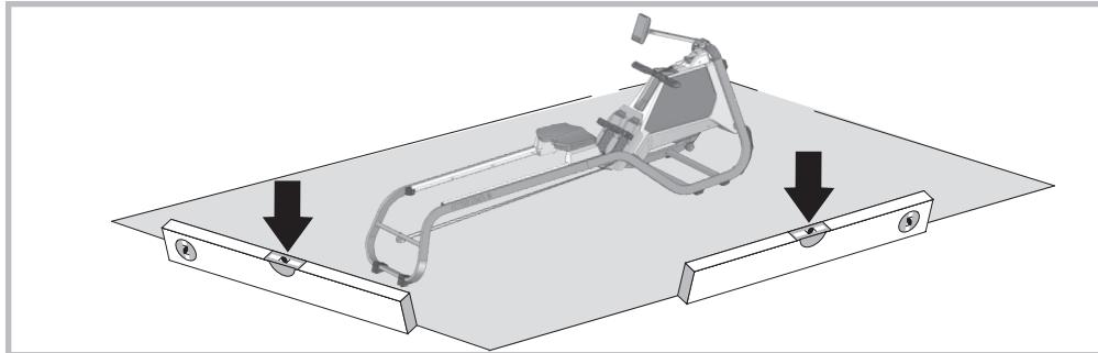
The location of the machine must be chosen so that sufficient safety distances to obstacles are ensured. It should not be set up in direct proximity to main walking directions. The free area must be at least 1 metre larger than the exercise area all around.
